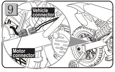
• Plug the motor connector into the vehicle connector.
