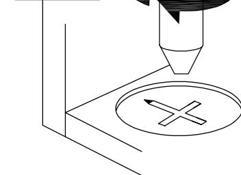
**EN** Turn cam lock clockwise to tighten.
