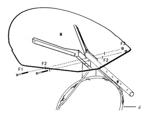
Insert top pole W into middle pole X, using bolt F.
