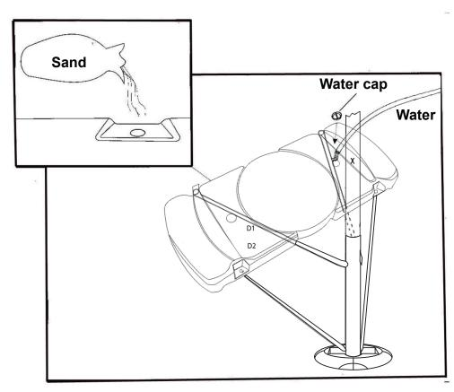
If the product does not need to be moved frequently, it is recommended to use sand in the base instead of water. Water could freeze, which damages the base. Please note, sand cannot be poured out after it is placed in the base.
