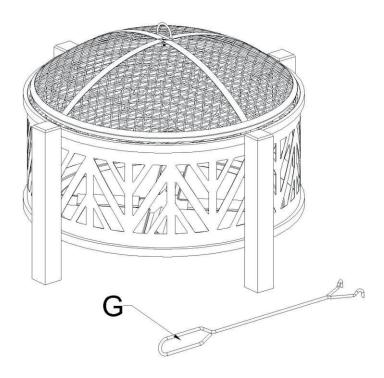
Before using, adda 1-1.5 in. layer of sand or about 10 lbs. (size wise, its the same amount as two 5 lb. bags of sugar) to the bottom of the firebowl.
