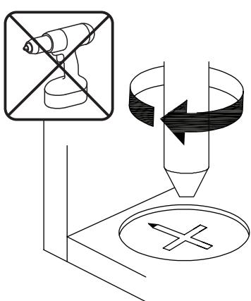
**EN**\_Turn cam lock clockwise to tighten.
