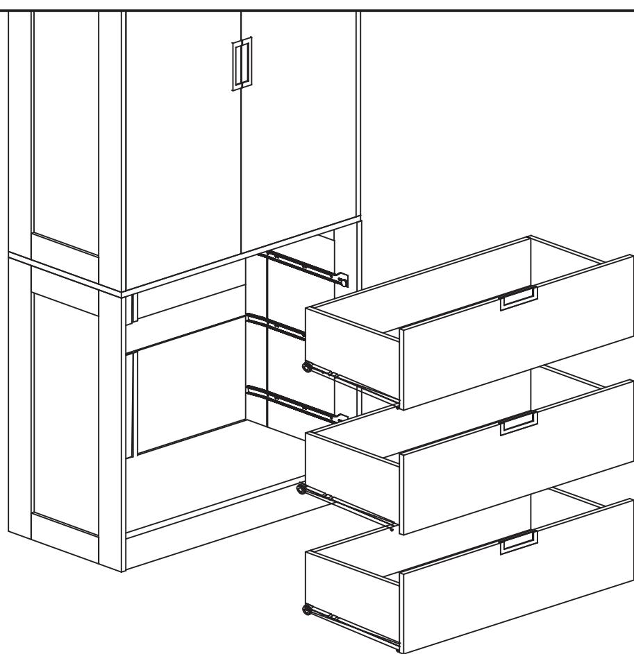
**EN** Be careful to push in the board when the both sides slide way been aligned.
