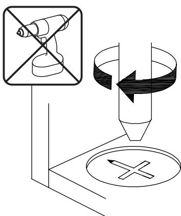
**EN** Turn cam lock clockwise to tighten.
