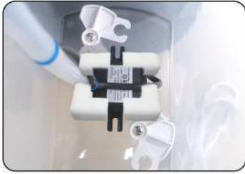
1. Remove the foam around the pump
