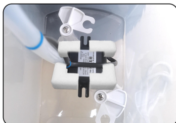
1. Remove the foam around the pump
