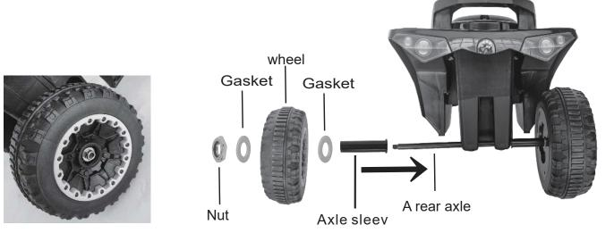
Installing the other side wheel is the same as step 1.
