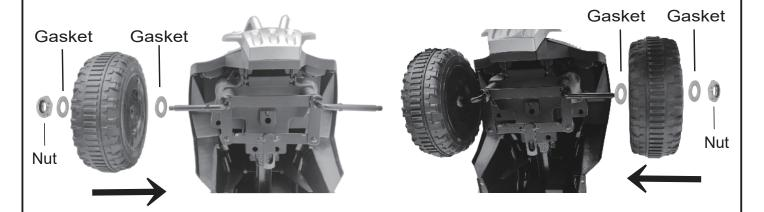
As shown by the arrow, pass the gasket, wheel, gasket and nut through the front axle and tighten the nut clockwise
