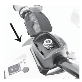
Insert the handlebar into the steering shaft, insert the gasket, and secure with a nut(M10\*1)
