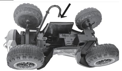
Turn the car upside down and insert the steering shaft
