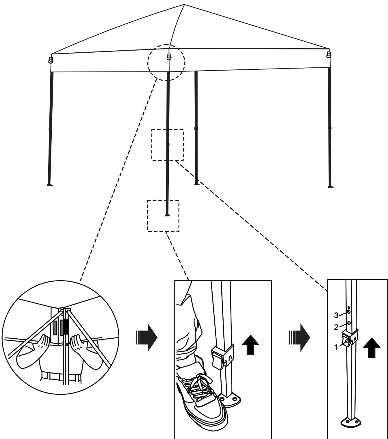
**EN** - There is a spring button on each leg for height adjustment.
