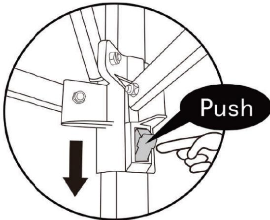
**EN** Push the push button on each slider to unlock the frame.
