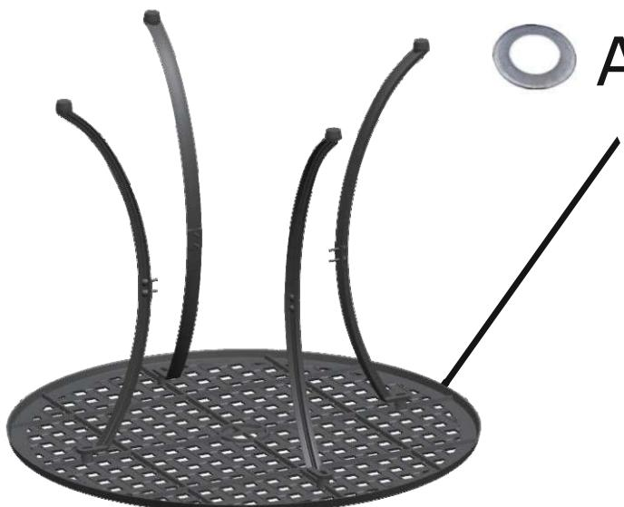
**EN** Attach the Table legs Support ((11))to the four Legs (10)using flat washer,spring washer and nuts(A,B,C) DO NOT over tighten.
