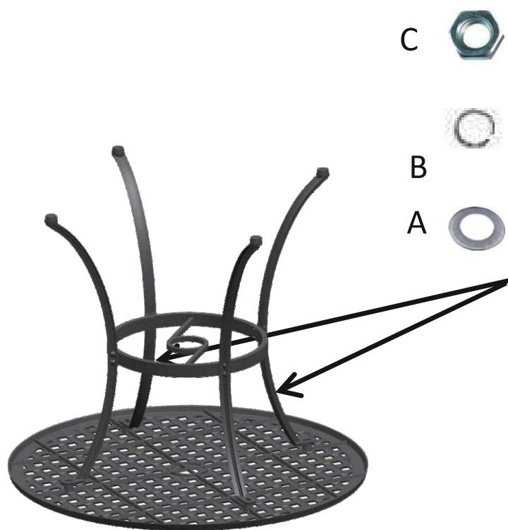
**EN** Tighten all nuts with wrench.And turn over the table.- Adjust the preinstalled rubber pad (l) until the table is level with the ground ,tighten all the nuts and cover them with nut Caps(j).Your table can use now.
