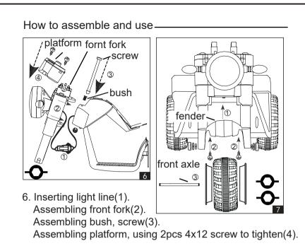
7. Assembling fender(1). Using 2pcs 4x12 screw to tighten(2). Assembling front wheel cover first, putting front wheel into fender, inserting front axle through front wheel(3), then one gasket each side, using screw to tighten.
