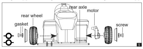
5. Assembling order to rear axle for left side is rear wheel, rear wheel cover, gasket, screw, for right side is motor, rear wheel, rear wheel cover, gasket, screw.
