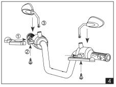
3. using 4pcs 4x12 screw to tighten.
