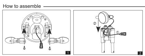
1. Assembling front light according to arrowhead, using 2pcs 4x12 screw to tighten.
