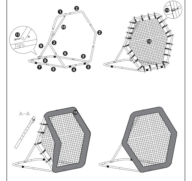
There are foot pad holes on the bottom part of net cover, please do not assemble in wrong position. The product must be assembled by adult.
