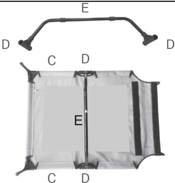
**EN** Connect the 2 centre plastic junctions D to the bed support leg E as illustrated. Then insert plastic junctions D into metal pipes C.
