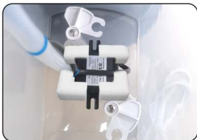
1. Remove the foam around the pump
