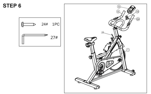
The Monitor Holder (10) is pulled and fixed on the Handle Frame (6) with the Self tapping screw (24) and tightened with the inner hexagonal wrench (27).
