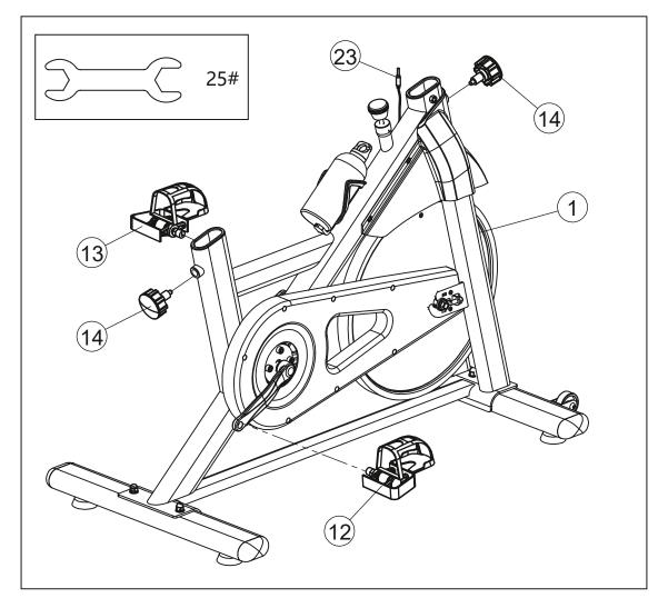
Install the right pedal (12) with R mark on The Main Body (1) and fix it with an open wrench (25). Note: tighten it clockwise.
