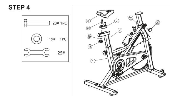
The Saddle Adjustment Frame (7) is installed in the Saddle Post (4) and fixed with the Flat washer (19), an six angle bolts (28) and a adjusting nut (15). Then the Saddle (8) is arranged on the Saddle Adjustment Frame (7), and is fixed and tightened with the open wrench (25). Install adjusting nut(29) on main body(1).
