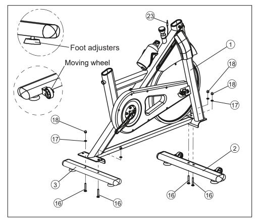
The Front Stabilize (2) is fixed on the Main Body (1) with Carriage Bolts (16), Flat washers (17) and cover nuts (18), and fixed with open wrench (25). Note: the move wheels of the Front Stabilize(2) are forward, as shown.
