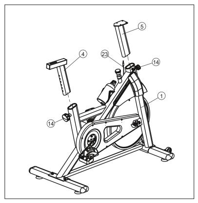
The Saddle Post (4) is inserted into the Main Body (1), and the Adjusting knob (14) is pulled out so that the Adjusting knob (14) is automatically inserted into the corresponding hole of the Saddle Post (4).
