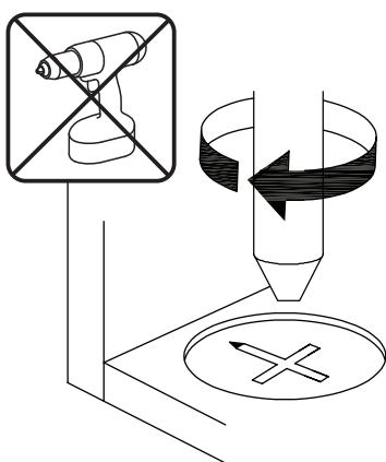
**EN** Turn cam lock clockwise to tighten.
