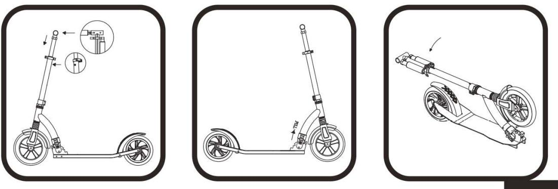
Loosen the upper lock, press the spring button and push down the T-bar to the lowest height. Tighten the upper lock to secure the T-bar. Press the spring button to release the handle from the T-bar and fix the handle on the grip bracket. Pull the folding button upwards and push the handlebar down until it clicks.
