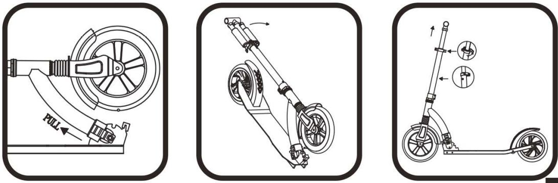
Push the folding button and pull up the handlebar until it clicks. Release the handle from the grip bracket and insert it into the T-bar, ensuring the spring button pops to secure it into its position. To adjust the T-bar, release the upper lock and press the spring button. You are now able to adjust the T-bar handle to three different levels, dependant on the user's height. Make sure the spring pops back into its hole and tighten the upper lock to secure the T-bar.
