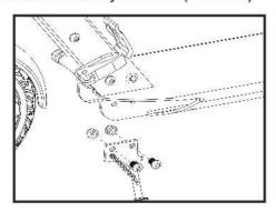
Step 2:Press the level of folding mechanism lock to loosen the transportation lock Push the handlebar stem until you hear it click into place.(Picture3)
