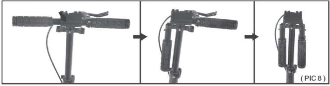
Step3: Pull the lever of quick release NO1 away the deck.
