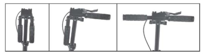
Step5: Loosen the quick release NO.2 lock on the handlebar stem by pushing the lever of the quick release lock until the lever is parallel to the handlebar grip.
