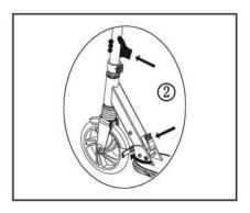
Step3: Fasten the quick release NO.1 (Picture4)
