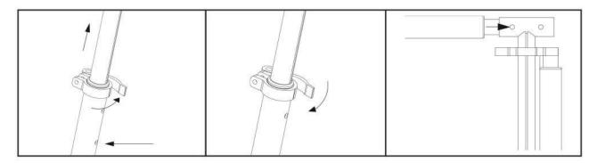
Step4: Insert the handlebar grips into the T- section of the handlebar stem. Use thumbs to press down both locking buttons until the grips can be easily pushed into the Fsection Turn the handlebar grips until the locking buttons are positioned in the two openings and hear them click into place(Picture 5)
