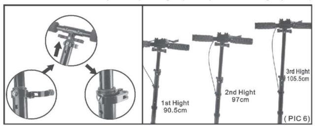
Always check all parts before use to ensure they are many uguary paradularly are rolling mechanism, the handlebar locking and the wheels
