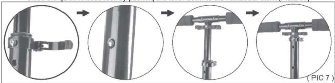
Step2: Use your thumbs to press both locking buttons in the handlebar grips and pull the handlebar grips outwards until they are released completely form the T-section.
