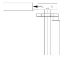
Loosen the quick lock and push forwards folding button, pull downwards tube. The scooter is folded completely when you sound clicks. Return back quick lock and ensure tighten it.
