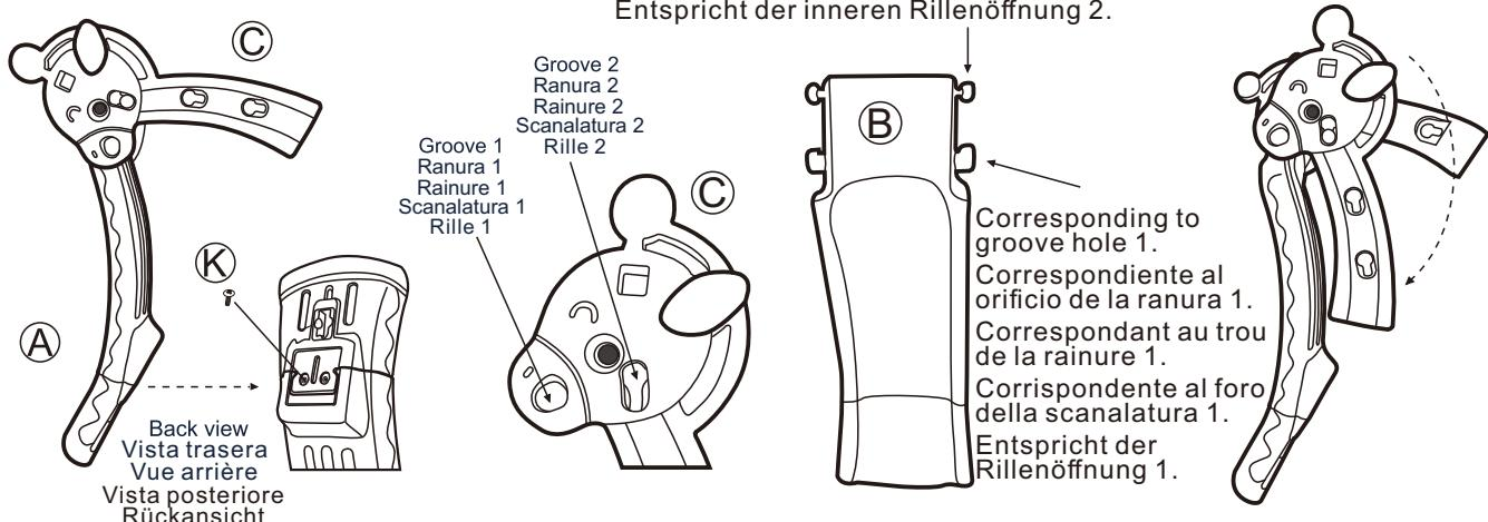
EN: Install slides and handrails. Twist the corresponding two groove holes of the slide rail to the armrest to the correct position.
