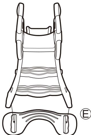
**EN:** Install the base. Press down on the corresponding groove hole.
