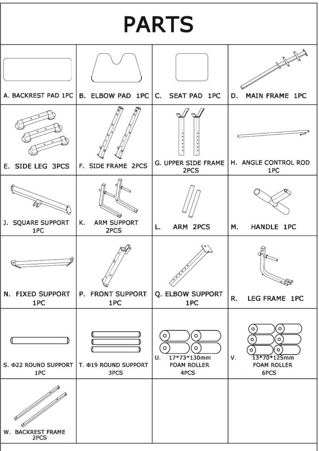
**REMARK:** PLEASE NOTE THE LEFT AND RIGHT DIRECTION BETWEEN **PART F** (SIDE FRAME) AND **PART K** (ARM SUPPORT) DURING INSTALLATION!
