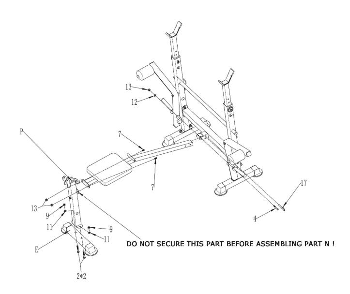
**Step7:** Attach part N fixed support to the main frame and front support with two part 5 screws.
