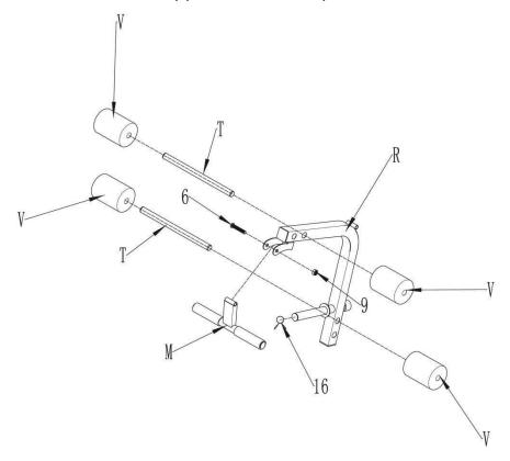
**Step9:** Attach the leg frame to the front support with a part 6 bolt and part 9 nut.
