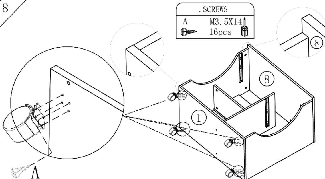
\* The bottom side of Panel #1 haven't preset holes for 4 wheels.
