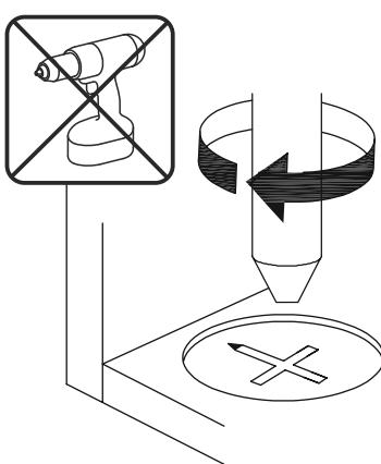
**EN** Turn cam lock clockwise to tighten.
