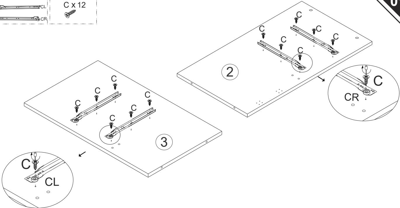
**EN** Please find the exact hole for installation, otherwise it will be misaligned. The screws on the drawer slide must be leveled , otherwise it will affect the smoothness of the d rawer.
