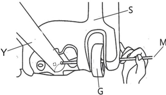
**EN:** Insert the wheel shaft (M) into the wheel (G), base (S) and end of the bottom pole (Y).
