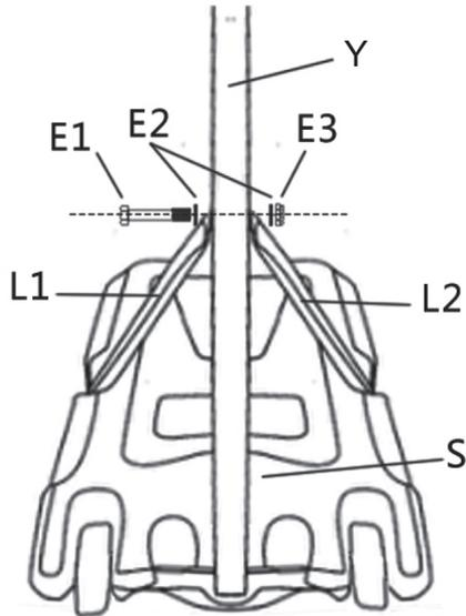
**EN:** Place one end of the pole brace (L1) & (L2) onto the bottom pole (Y), using the bolt set (E1), (E2) & (E3).
