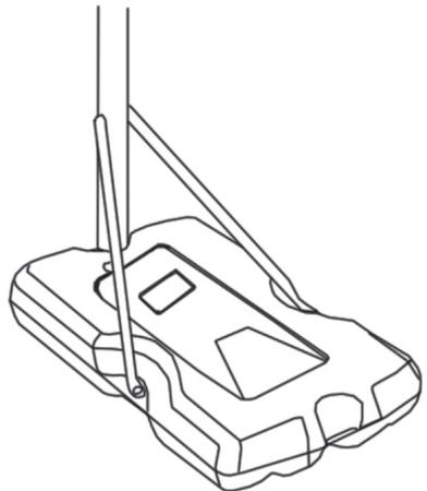
**EN:** Place the other end of the pole brace (L1) & (L2) onto two sides of the base (S), using the bolt Set (C1), (C2) & (C3).
