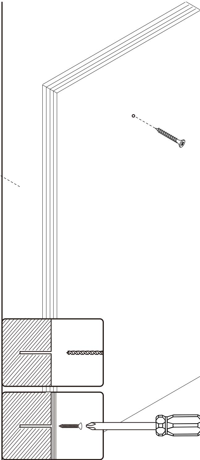
**EN** If it is a solid wall, please use expansion and self-tapping screws, if it is a wooden wall, only use self-tapping screws, please do not overtighten the screws
