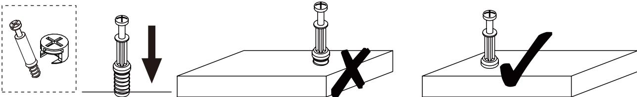
**EN\_QUICKFIT:** Tighten quickfit until shoulder is flush with panel. Do not overtighten or undertighten.
