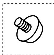
**EN** Adjust up and down for balance
