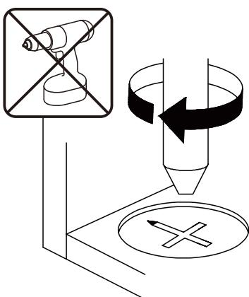
**EN**\_Turn cam lock clockwise to tighten.
