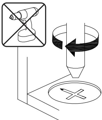
**EN**\_Turn cam lock clockwise to tighten.
