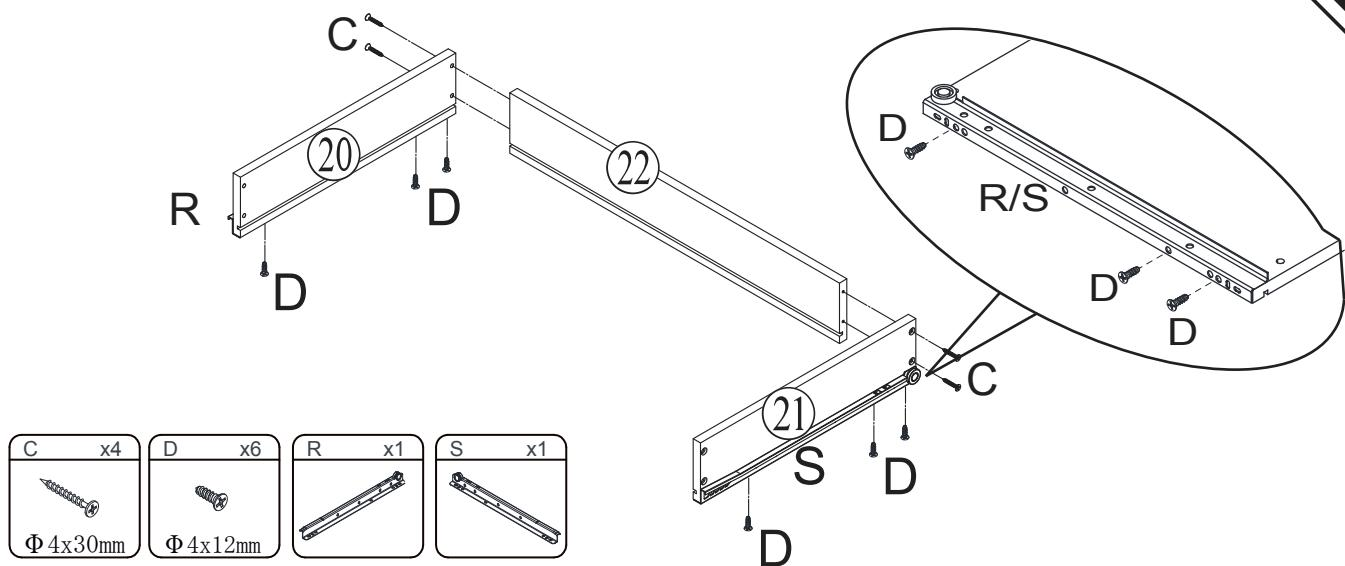
**EN** Please find the exact hole for installation, otherwise it will be misaligned. The screws on the drawer slide must be leveled , otherwise it will affect the smoothness of the drawer.
