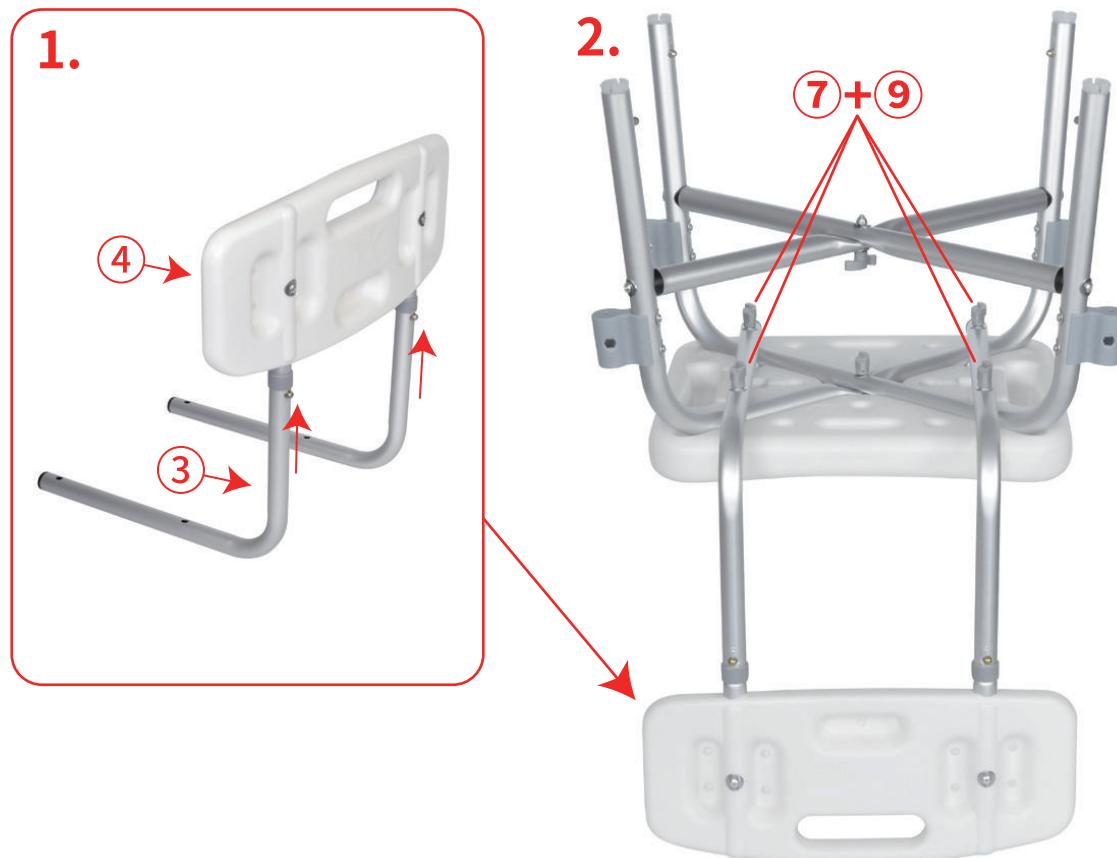
**EN**\_1.Insert the backrest tube③\*2 into the backrest board④ till the marble is secured
