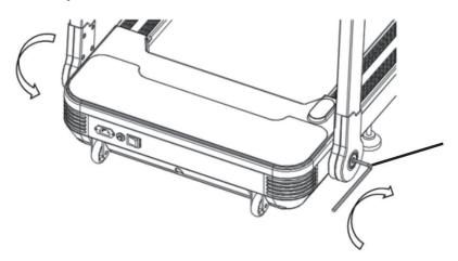
Step3 Use the 6# Allen wrench to lock the screws which is inside the both decoration covers in clockwise direction.( If the handles can be shaken easily, please keep locking the screws)
