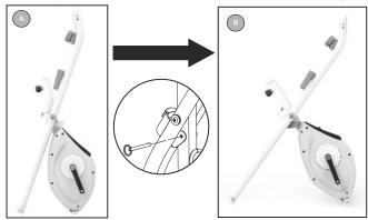
2. Please assemble the front and back support frames in order. The front and back support frames can be distinguished install the frame with wheels on the front. Fasten the nuts and washers on the support frame using a small wrench.
