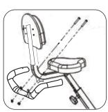
5. Installation of the LCD monitor and handle. Please connect the monitor to the groove of the lower main body and tighten the screw with an allen wrench.
