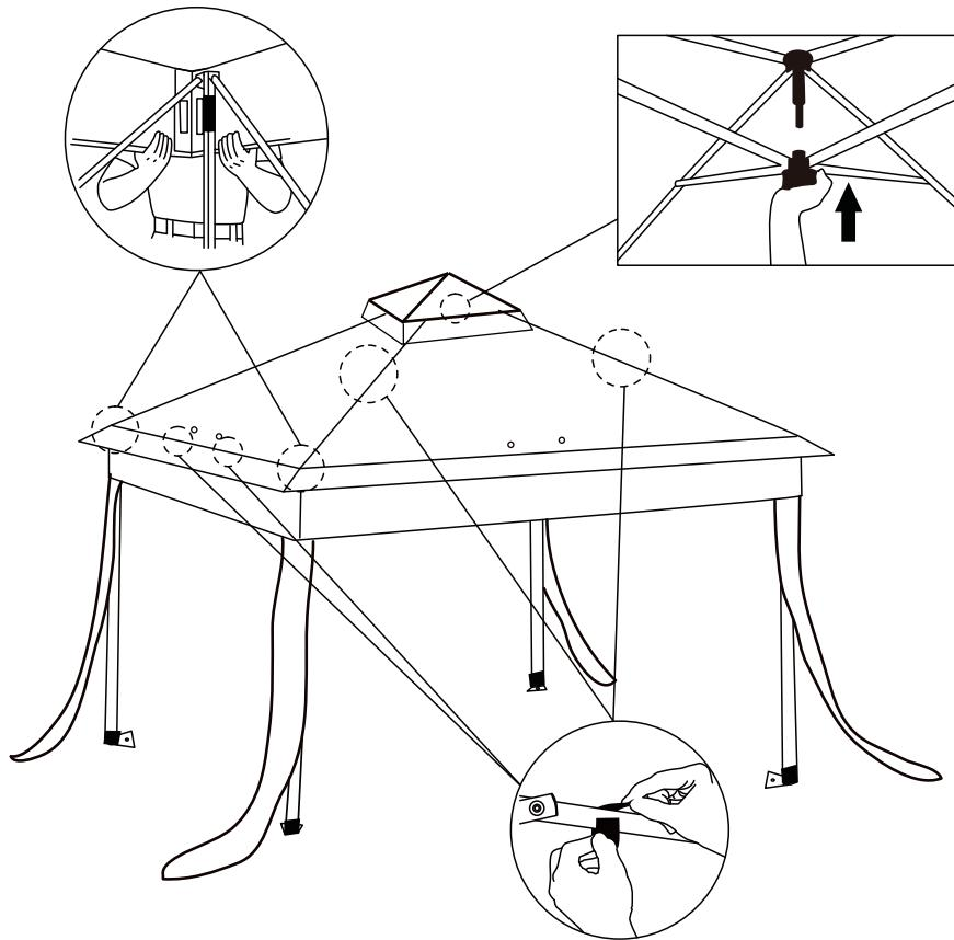
**EN** Attach the canopy fabric to the frame with the loop fasteners. Push up the central locking system until it locks into place and the entire frame is fully extended. After setting up the canopy fabric. Please reinforce the fabric to the frame with the loop fasteners inside the canopy.
