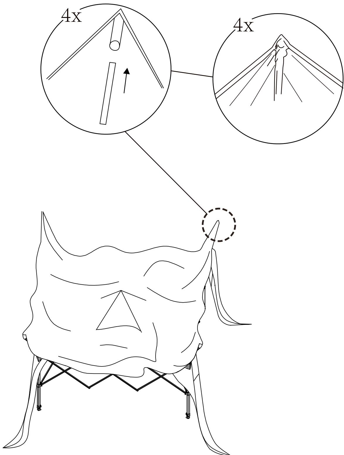
**EN** Install the four corners of the fabric onto the pipes at the four corners of the bracket.
