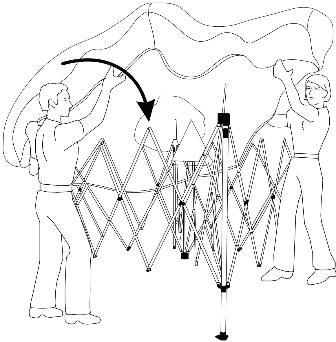
**EN** Place the canopy fabric on the frame and align the four corners of the canopy fabric with the four corners of the frame.
