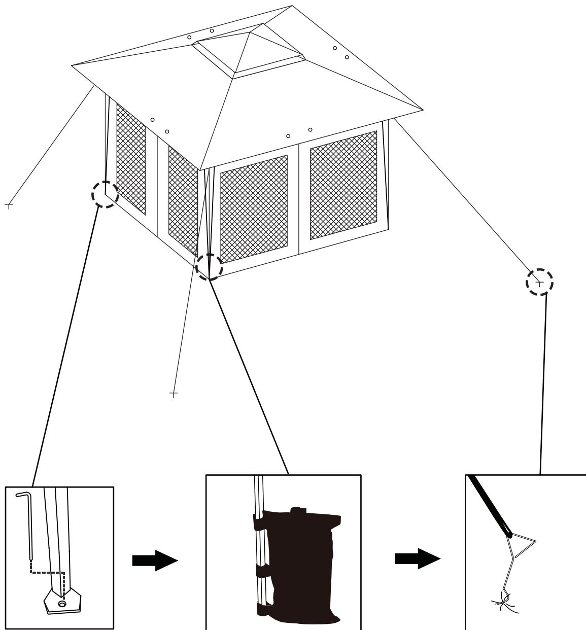
**EN** Connect the canopy fabric and the ground anchors with ropes, and fix the anchors into the ground for added stability.
