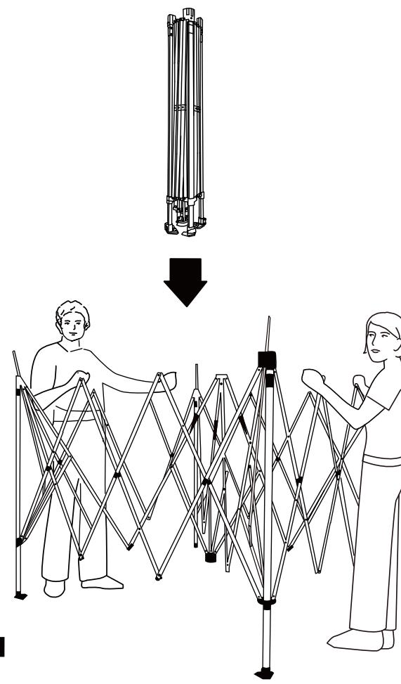
**EN** Erect the frame and half open it.
