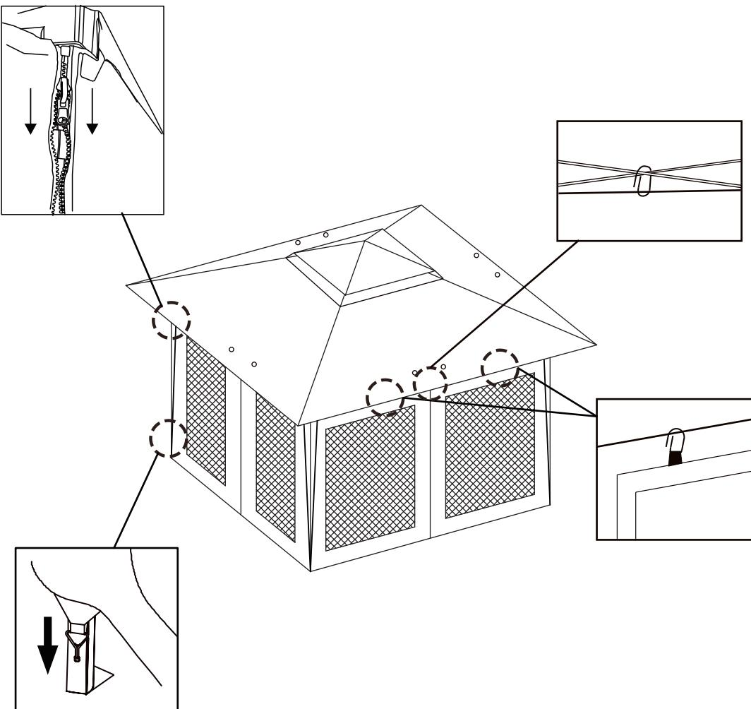
**EN** When assembling, please completely attach the of the wall as well as the door to the canopy fabric of the top before zipping the walls down.
