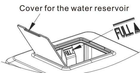
Warning: Do not pour water into the internal tank underneath the ice basket. The tank is too small and will affect the machine's performance.
