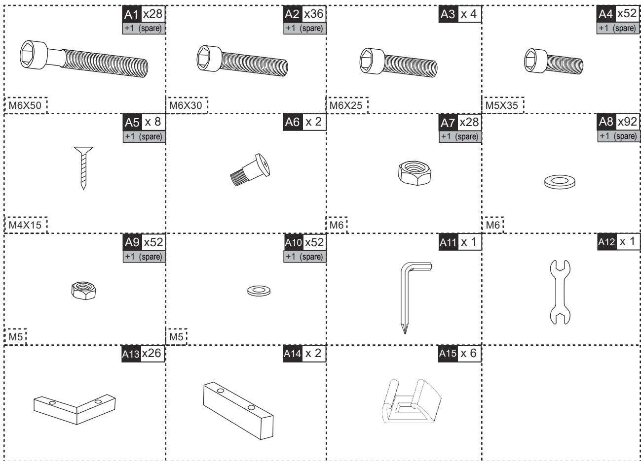
**EN** Do not confuse similar screws. Do not tighten bolts fully until all parts are connected!
