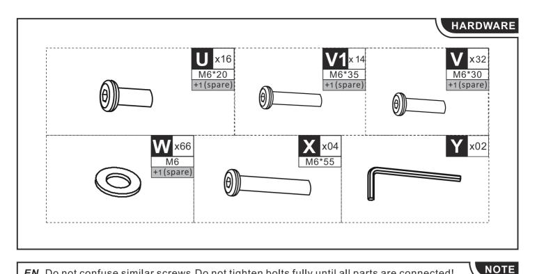
**EN**\_Do not confuse similar screws.Do not tighten bolts fully until all parts are connected!
