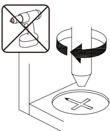
**EN** Turn cam lock clockwise to tighten.
