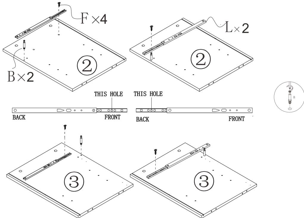
**EN** Please find the exact hole for installation, otherwise it will be misaligned. The screws on the drawer slide must be leveled , otherwise it will affect the smoothness of the d rawer.
