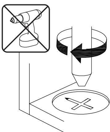
**EN**\_Turn cam lock clockwise to tighten.
