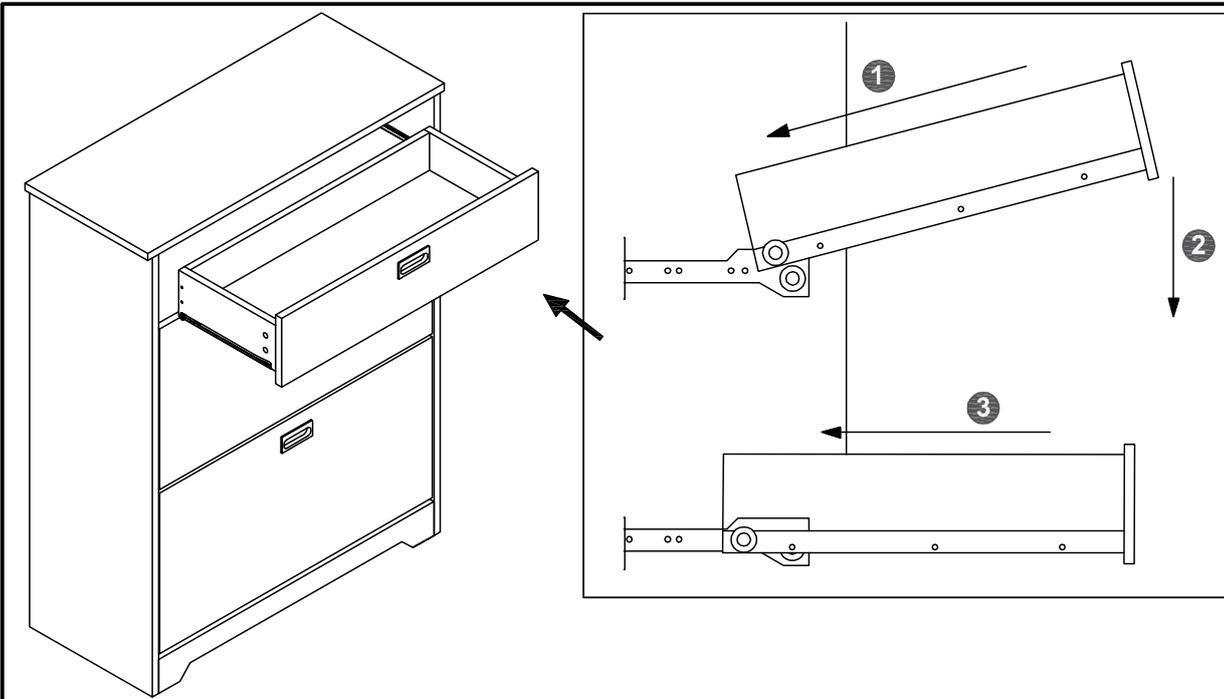
**EN** Be careful to push in the board when the both sides slide way been aligned.
