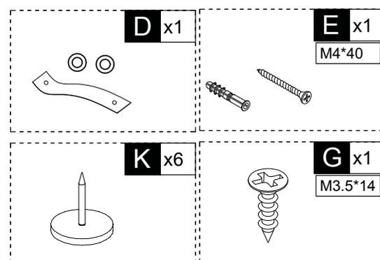
**EN\_** If it is a solid wall, please use expansion and self-tapping screws, if it is a wooden wall, only use self-tapping screws, please do not overtighten the screws
