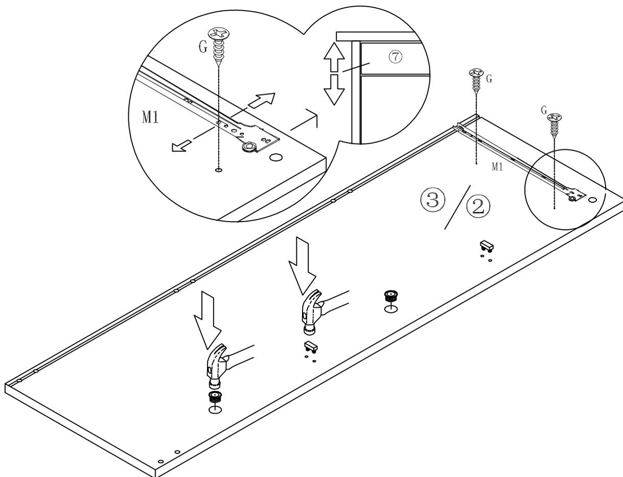
**EN** Please find the exact hole for installation, otherwise it will be misaligned. The screws on the drawer slide must be leveled, otherwise it will affect the smoothness of the drawer.
