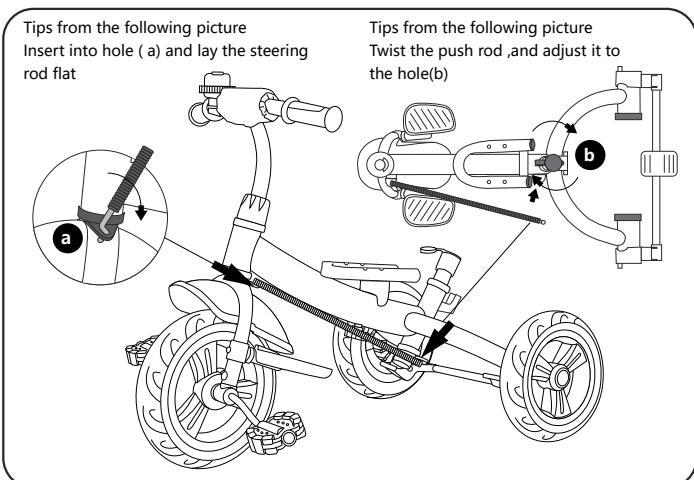
4. As shown in the picture, first insert the front wheel assembly into the main frame, then fit the front cover into the handlebar opening, and then insert the handlebar opening into the fork's upper opening, aligning the fork screw hole with the handle screw hole. Insert the handlebar fixing screw through the opening; then, using a socket wrench, tighten it and lower the front cover. Finally, install the bell on the handlebar.
