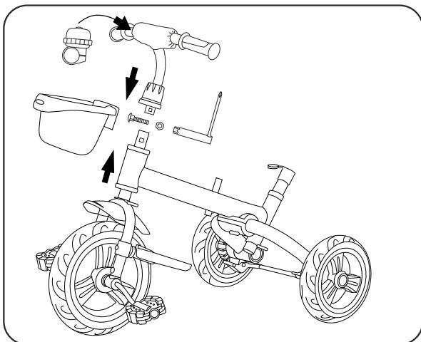
4. As shown in the picture, first insert the front wheel assembly into the main frame; then fit the front basket, and then fit the front cover onto the handlebar tube, then insert the handlebar tube into the front fork upper tube, aligning the front fork screw hole with the handlebar screw hole. Insert the handlebar fixing screws through the tube hole; then use a socket wrench to tighten them, lower the front cover; finally, install the bell on the handlebar.
