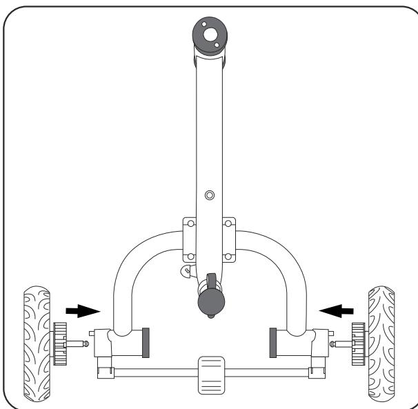
1. As shown in the picture, insert the rear wheel axle into the main frame rear dropout, gently tap until it locks with a "click" sound.
