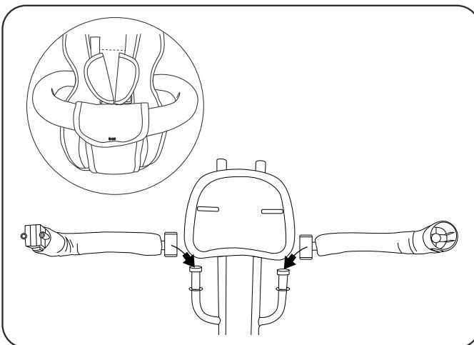
8. As shown in the picture, slide the left and right parts of the frame down along the groove of the slot, and then thread them through the front bar of the seat cushion cover, close the left and right frames.
