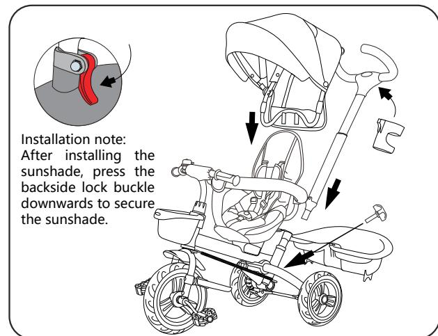
9. As shown in the picture, first insert the push rod into the connecting tube at the rear of the seat until it locks with a "click" sound, completing the lock. Hang the bottle holder; then align and insert the canopy tube into the backrest tube and lock it; finally, position the basket properly and secure it with the basket fixing knob.
