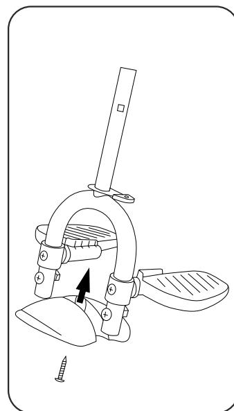
2. As shown in the picture, fix the front fender to the front fork with screws (crescent-shaped groove facing forward).
