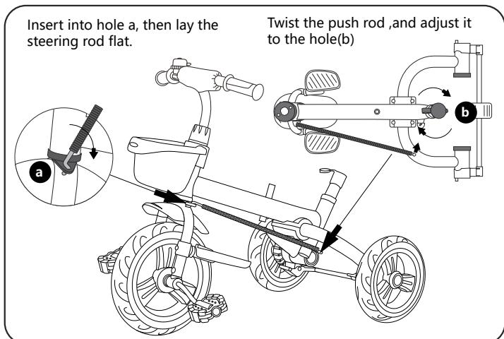
5. As shown in the picture, first unscrew the nut at the rear end of the steering rod, then insert the front end of the steering rod vertically into the front fork hole a, lay the steering tube flat, ensuring a secure connection with the front fork hole; twist the lower push tube to adjust push tube hole b so that the rear end of the steering rod can be hooked into the hole; once hooked, tighten it with a nut.
