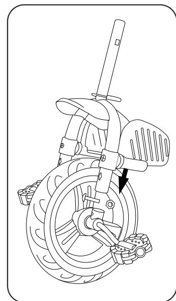
3. As shown in the picture, first insert the headset into the front fork and secure it with bolts and nuts.
