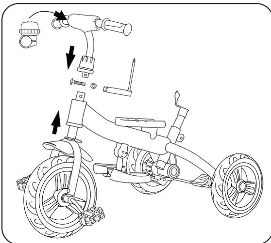
4. As shown in the picture, first insert the front wheel assembly into the main frame, then fit the front cover into the handlebar opening, and then insert the handlebar opening into the fork's upper opening, aligning the fork screw hole with the handle screw hole. Insert the handlebar fixing screw through the opening; then, using a socket wrench, tighten it and lower the front cover. Finally, install the bell on the handlebar.
