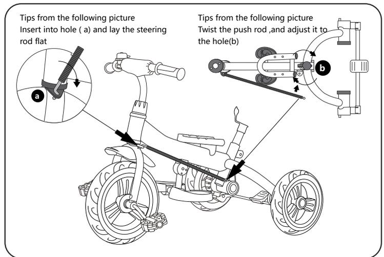
5. As shown in the picture, first unscrew the nut at the rear end of the steering rod, then insert the front end of the steering rod vertically into the front fork hole a, lay the steering pipe flat, ensuring a secure connection with the front fork hole; twist the lower push tube to align the push tube hole b so that the rear end of the steering rod can be hooked into the hole; once hooked, secure it with a nut.
