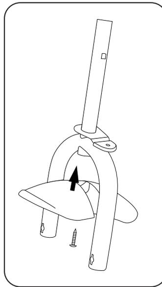
2. As shown in the picture, fix the front fender onto the front fork using screws.
