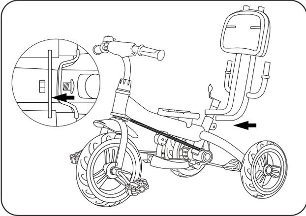
6. Insert the guardrail bracket into the seat tube and secure it with screws.
