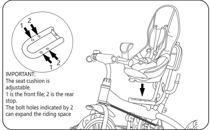
7. Align the seat with the frame screw hole and secure it with screws.
