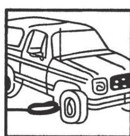
When using a jack, always centre it under the axle or a flat reinforced frame surface. This ensures proper stability and support during lifting.
