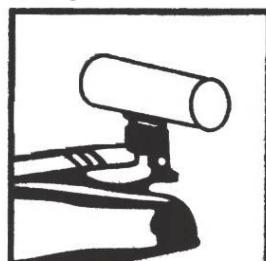
For the most stable support, ensure the load is always placed at the centre of the jack's saddle.
