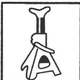
Before starting any work or inspection on a vehicle, ensure the weight is adequately supported by jack stands rated at the appropriate capacity.
