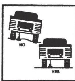
Only use this jack on hard, level and stable surfaces. Using it on uneven surfaces may lead to instability and a potential failure to support the load.
