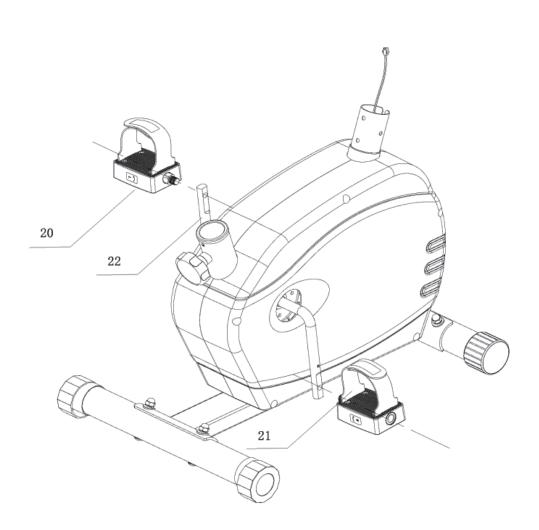
Attaching the pedals to the crank assembly:
