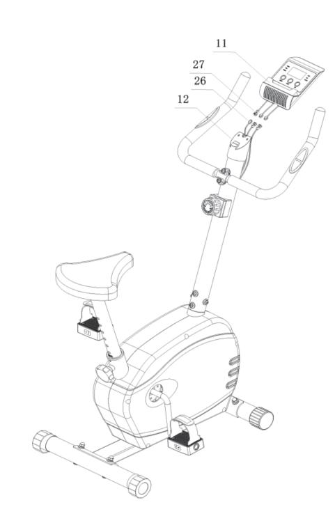
Connecting the sensor lines and the electronic watch:
