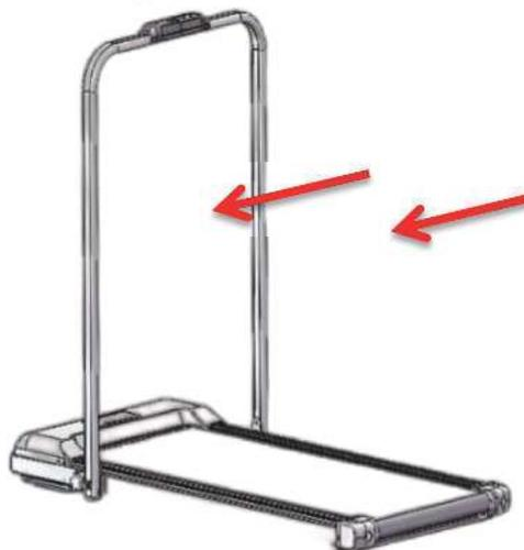
Step 4. To install the mobile phone support, position it above the armrest and align it with the hole. Insert it into the buckle until it securely snaps into place.
