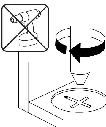
**EN**\_Turn cam lock clockwise to tighten.
