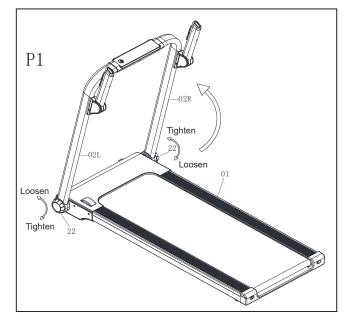
STEP1: Unscrew the knob(22)anti-clockwise about 4round,then follow the direction of arrow to unfold the post(02L/02R),finally,secure the knob(22)clockwise until its tightened.
