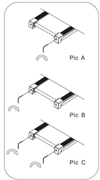
If the belt has drifted to the right, unplug the safety lock and power switch, and turn the right adjusting bolt 1/4 turn clockwise, then insert the power switch and safety lock, re-start the treadmill and observe the running belt to see if it deviates. Repeat the above steps until the running belt is aligned in the middle. See picture A
