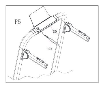
STEP4: Put safety key(35)on monitor(08)as pic5
