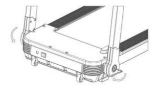
3. Take out the inner hexagon spanner(#6) from spare kit , put one end of the spanner into the screw hole of decorative cover ,tighten the screw in clockwise direction . the same installation method to the other end .(Loosen the screws in anticlockwise direction when dismantlement needed ).
