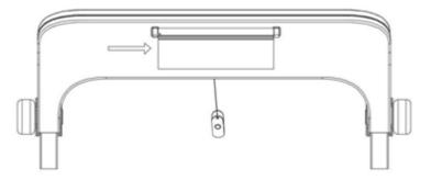
6. Turn the mobile holder upward after pushing the mobile holder to the right side ( as the arrow shows ) until the holder is free from the slot.
