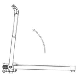
2. Raise the standpipe or Meter Asy and turn it to the direction as the arrow shows , until It stands still .
