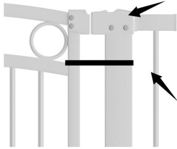
The door gap is NOT a defect! after installation, it will be shortened to 0.2cm
