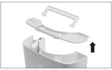
Dismount the water tank for cleaning and remount it in the reverse way before reinstalling it to the appliance
