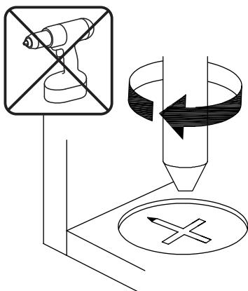
**EN**\_Turn cam lock clockwise to tighten.
