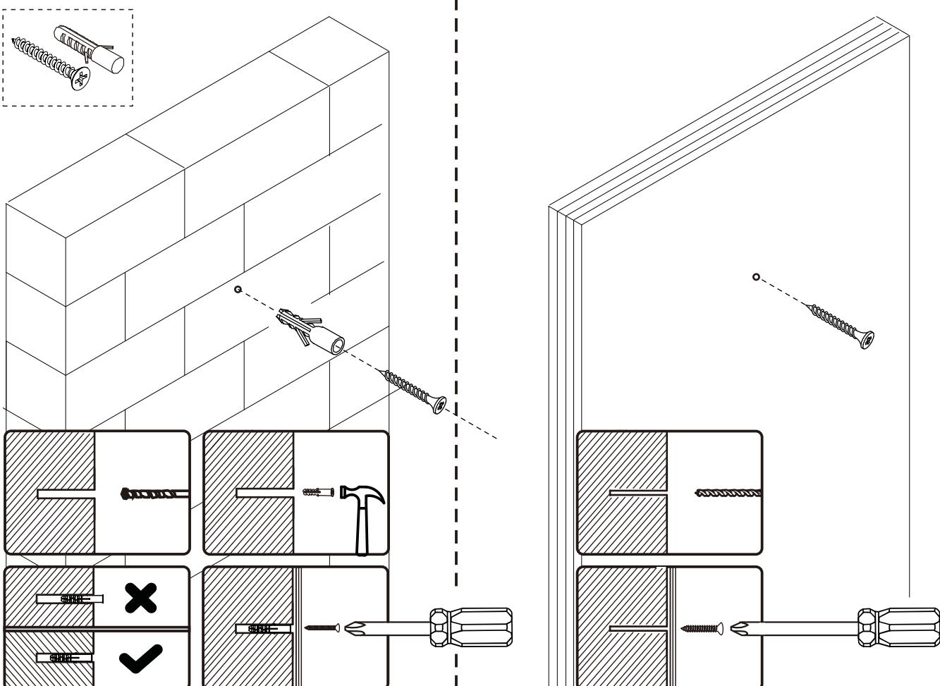
**EN** If it is a solid wall, please use expansion and self-tapping screws, if it is a wooden wall, only use self-tapping screws, please do not overtighten the screws
