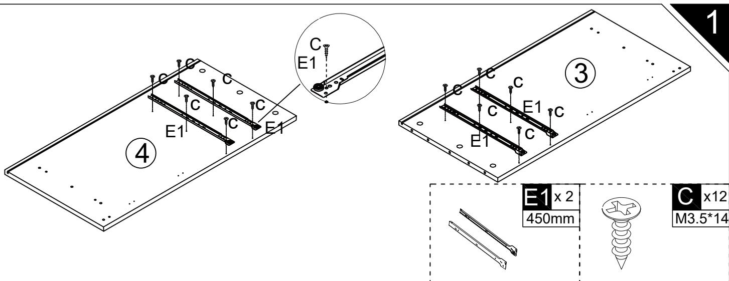
EN\_Please find the exact hole for installation, otherwise it will be misaligned. The screws on the drawer slide must be leveled , otherwise it will affect the smoothness of the drawer.
