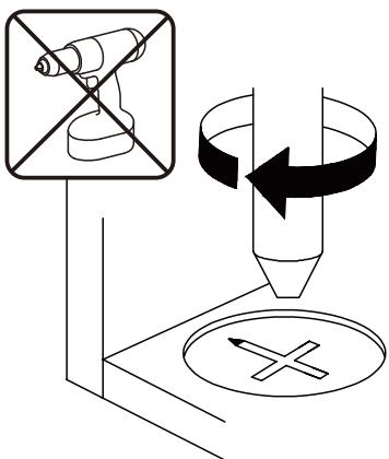
**EN**\_Turn cam lock clockwise to tighten.
