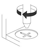
**EN** Turn cam lock clockwise to tighten.
